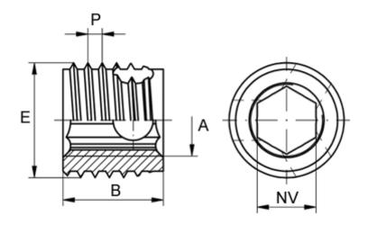
Female thread A = M4= 8 Length B Male thread E = 6.5Min hole depth blind hole = 10 Min material thickness = -SW
